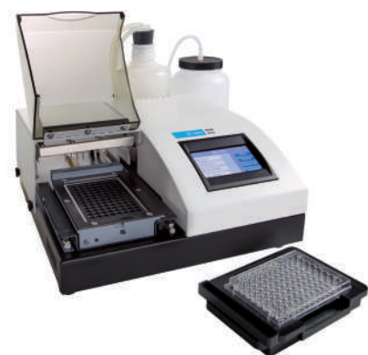
Figure 2. Wash filter-bottom plates and magnetic bead assays with available modules.
